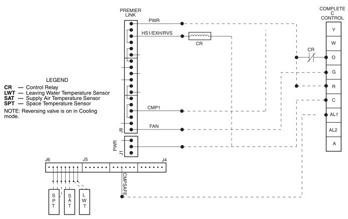
Fig. 7 — PremierLink Controller Applications with Complete C Control
